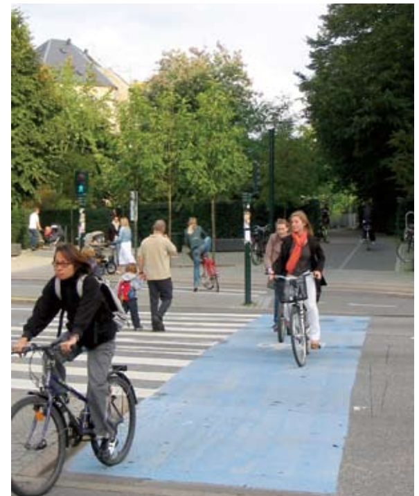
Intersection treatments ensure that routes and paths are continuous, cyclists know where they should ride, and drivers and pedestrians have clear signals of when and where to expect cyclists.
